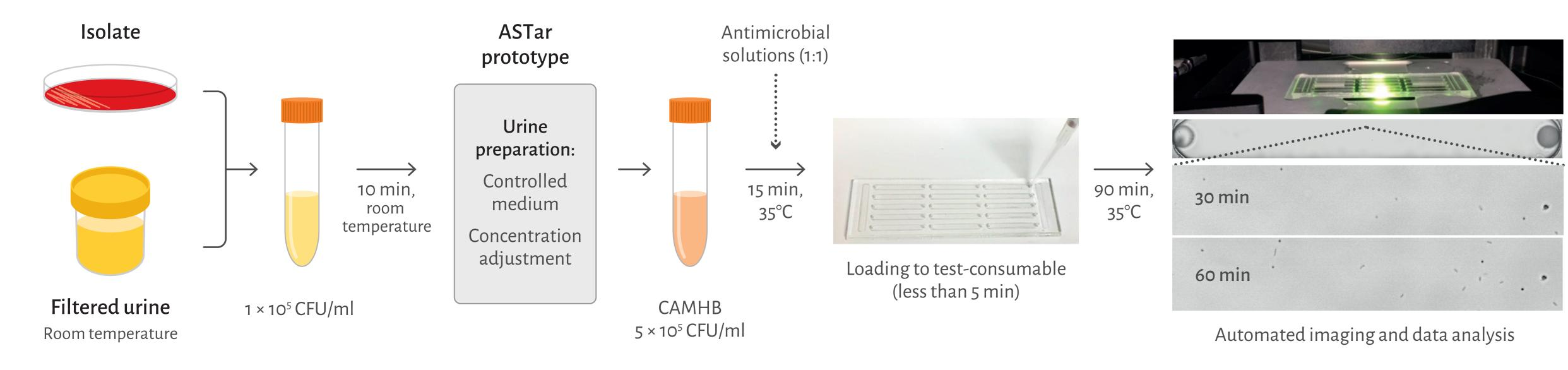
Fig 2. Experimental set-up.
