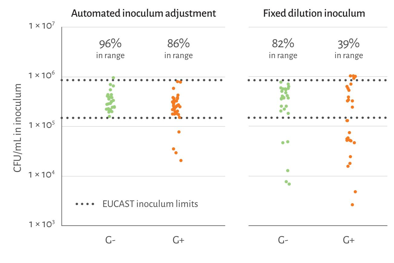
Fig 2. Comparison between inoculum concentrations achieved using ASTar automated sample processing compared with what would have been achieved using fixed dilution for gram-negative (G-) and gram-positive (G+) organisms.
